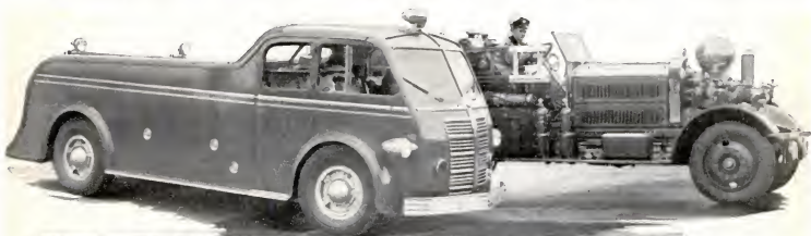
New-type fire engine contrasted with one of conventional design. Six firemen can ride in the roomy, air-conditioned cab in front
